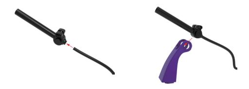
Insert the air pipe through the upper and lower holes of the launch pad in sequence.
